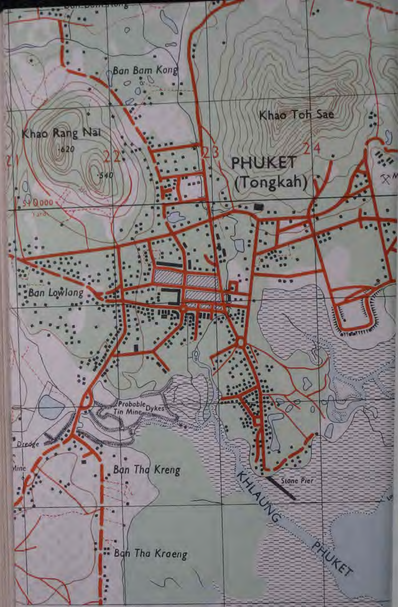
Plate 26. Siam. 1:25,000. "Phuket Island." Compiled from air photographs, using Multiplex projectors, by 653 Eng Bn U.S.A.A.F. (Feb. 1945.)
